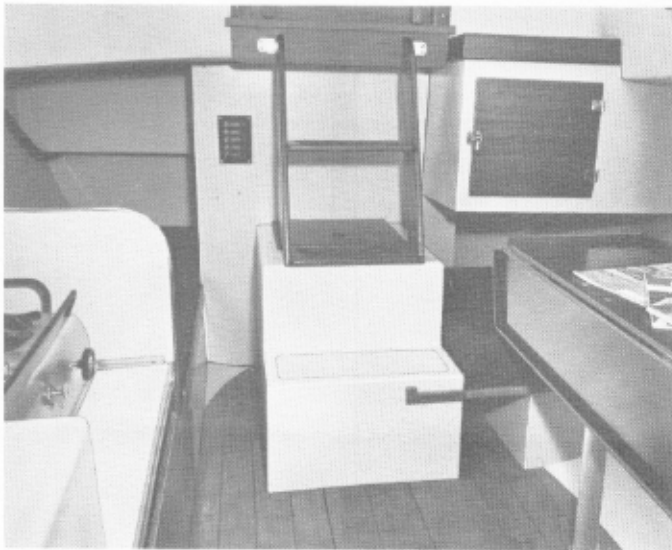
Looking aft in the main cabin one sees the quarter berth on the starboard side, the fully enclosed motor compartment with its easy access, a corner of the dinette above which shows the interior access door to the food storage compartment of the ice box.
