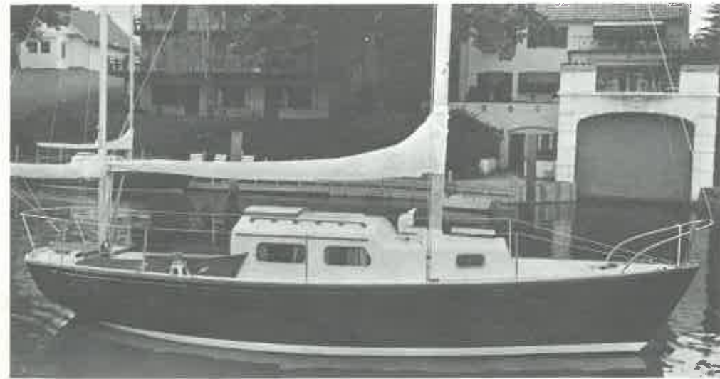
TARTAN 27 may be had sloop or yawl rigged. The modern masthead rig permits carrying the generous sized headsails so desirable in racing. The yawl provides for an easy rig to sail, when cruising short handed.
